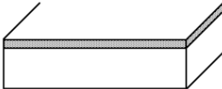
1. Cover wafer with masking material
